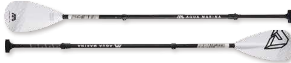
SOLID Fiberglass iSUP Paddle SHAFT: 1.25mm thick 100% fiberglass. Diam: 1.13" (28.7mm). BLADE: 60% PP + 40% fiberglass. L x W: 15.7" x 8.7" (40 x 22cm). HANDLE: Rubber T-bar handle. LENGTH: 70.9"-86.6" (180-220cm), 3PCS adjustable. WEIGHT: 950g (33.5oz)
