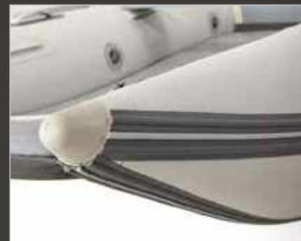
The high quality anti-collision rubber strake will get the boat well protected when there is an impact.
