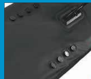
1+8 or 1+16 self-bailing drain valves that can be left open in whitewater and ocean kayaking conditions
