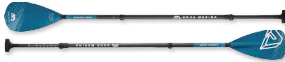
CARBON GUIDE Carbon/Fiberglass iSUP Paddle SHAFT: 1.25mm thick 70% carbon + 30% fiberglass. Diam: 1.13" (28.7mm). BLADE: 60% PP + 40% fiberglass. L x W: 15.7" x 8.7" (40 x 22cm). HANDLE: Rubber T-bar handle. LENGTH: 70.9"-86.6" (180-220cm), 3PCS adjustable. WEIGHT: 950g (33.5oz)
